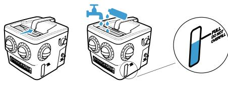
No damage will result if the unit is used without water -- When using in a moving vehicle, only half fill and secure unit Only half fill with water when using ice -- When adding ice, keep ice level below bottom of vents inside the unit If using external water tank situate it at a higher level than the E3 unit to allow water to gravity feed into unit via hose
